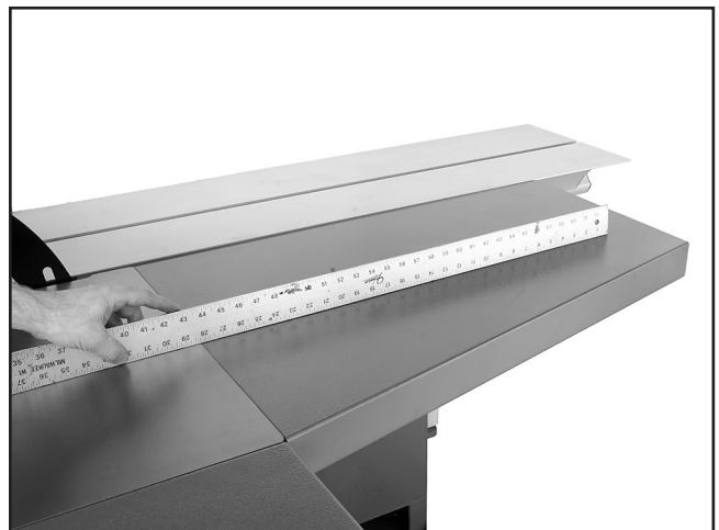
Figure 22. Checking with a straightedge.
